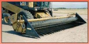
Pans guide stalks into the header's cutting bar while greatly reducing shelling loss.
